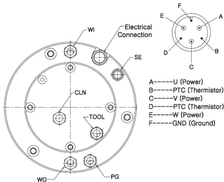
WI-----Cooling Water IN (1/4 x  $\phi 10\text{mm}$ )
